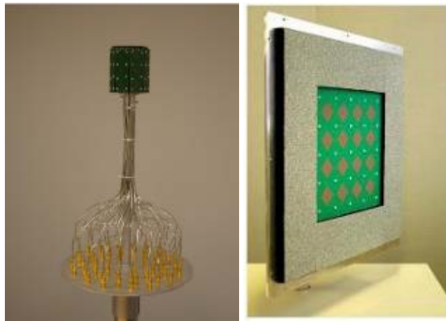
Figure A1.2.1-1. Omni-directional antenna array (ODA) at left (receiver), Uniform planar antenna array (UPA) at right (transmitter)
